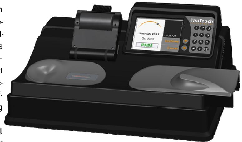
The light used in the TruTouch measurement is in the near-infrared (NIR) and is safe for human skin exposure. The light levels are less than the limits established by the FDA for non-ionizing radiation ("orders of
