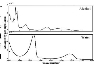
Figure 1 - NIR absorptivity of alcohol and water
